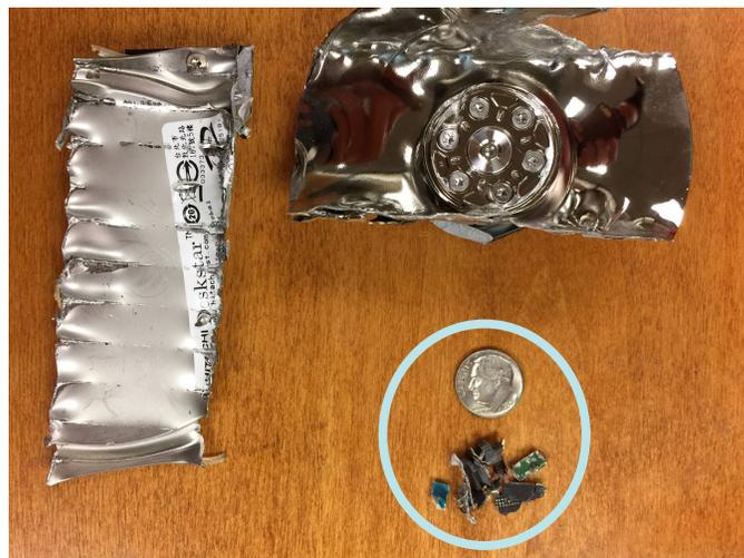
Compare a regular hard drive shredded in the traditional manner at 1-1/2" strip shred, to our SSD Micro-Shredder shredding at less than 3/16th of an inch.
