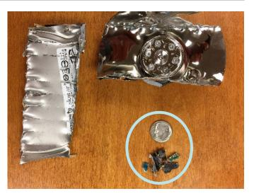
Compare a regular hard drive shredded in the traditional manner at 1-1/2" strip shred, to our SSD Micro-Shredder shredding at less than 3/16th of an inch.
